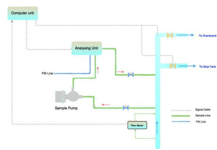
Cleaning line and sample lines into the measuring cells are segregated by pneumatic valves. So when cleaning cycle is initiated following takes place
