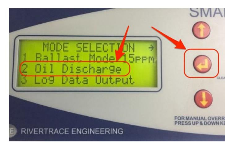
Under "Oil Discharge Set Up", go to "alarm limit" and press enter.
