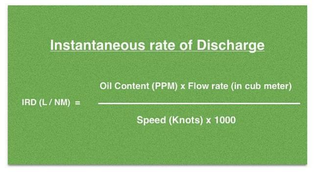
Now if ODME need to measure IRD, it surely need values for oil content in PPM and Flow rate. Speed connection is usually given either from log or GPS.
