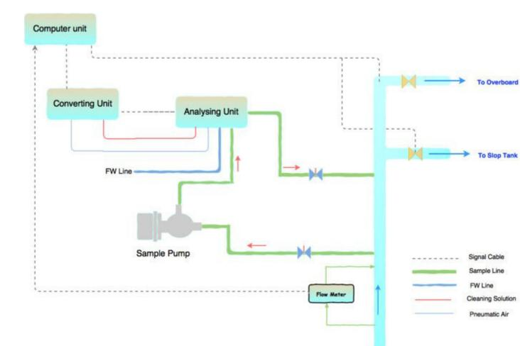
The computing unit also calculates the amount of actual oil that has been discharged to sea. The requirement is that we cannot discharge total oil more than 1/30000 of the total cargo carried. Before we start ODME, we need to calculate and feed this maximum allowed value in the ODME. This we will discuss later in this post.
