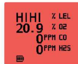
Red display in alarm conditions
